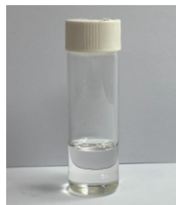
■ Our PbBr 2 can readily be dissolved in DMF to yield 1M solution.
